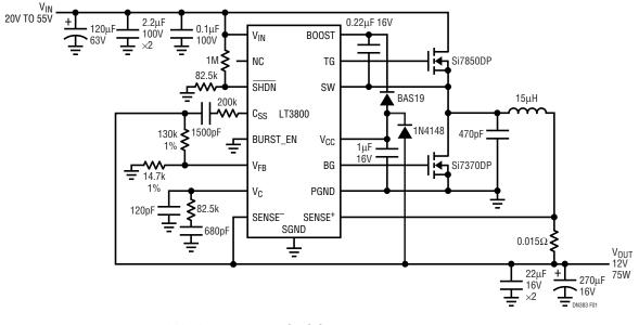
Figure 1. LT3800 12V, 75W Buck DC/DC Converter with High Efficiency at Light Loads
