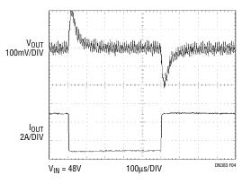
Figure 4. 1A to 5A Load Step Generates <2% V<sub>OUT</sub> Transient
