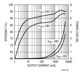
Figure 2. The DC/DC Converter in Figure 1 Exhibits High Efficiency Across a Wide Load Range and Produces Peak Efficiencies Above 95%
