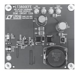
Figure 5. LT3800 12V, 75W DC/DC Converter Layout
